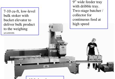
Allen-Bradley PLC based Control Instrument with PanelView touchscreen
