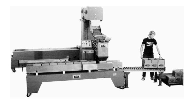
System Shown: **Delta Model LWSK9 with 1SK Box Conveyor and C Bucket Loader**
