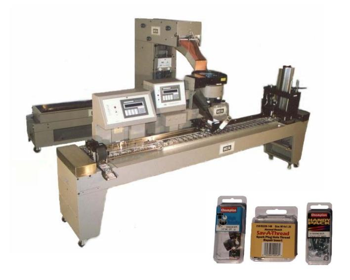
A fully automated system for dispensing, filling, and closing one-piece, hinged-lid, plastic display boxes.
